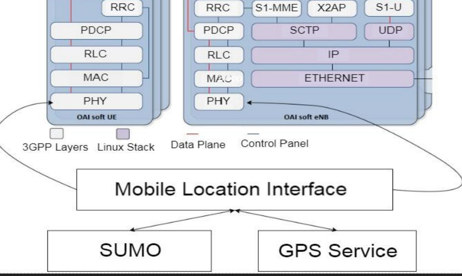
Interface interacts between SUMO and OAI/GPS system. Mobile Location Interface sends location data to MAC or PHYS layer of the OAI eNB and UE. The PHYS layer encodes/decodes the packets and MAC layer handles
