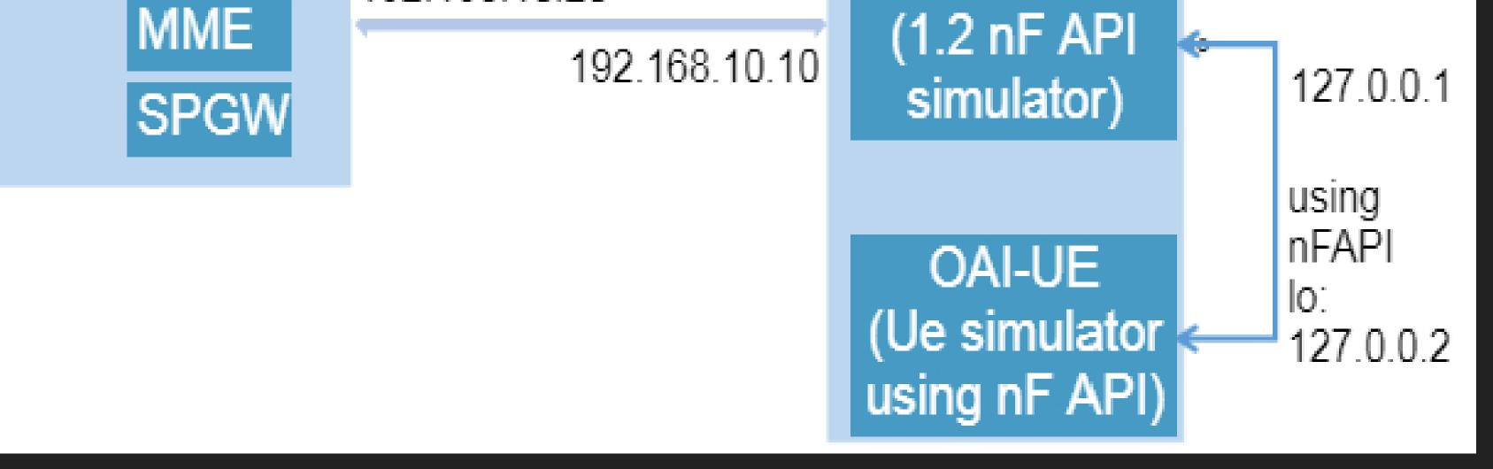
ENB and UE run on a single system (shown on the right), and are connected by nFapi using loopback IP interface. OAI allows us to conduct purely software-based network simulations and eventually deploy the network to physical hardware.
